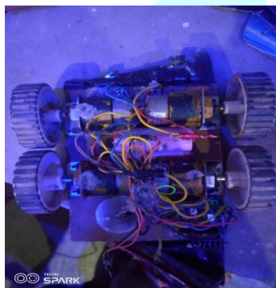
Installing the Motor and battery on the Robot
