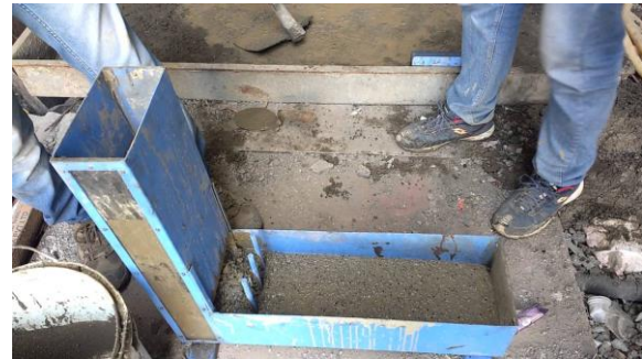
Fig 7: L Box Test Apparatus
