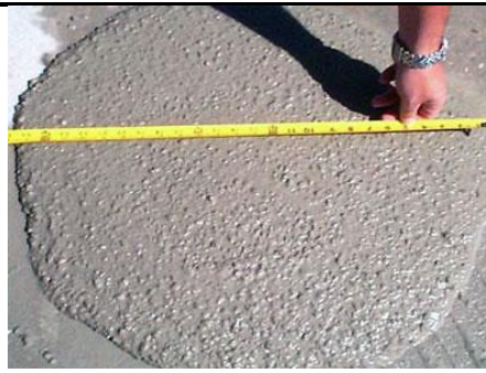
Figure 6: Slump flow test at field
