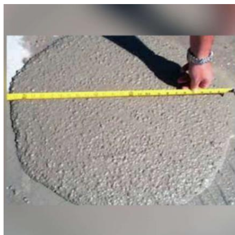
Figure: T50 Slump Flow Test
