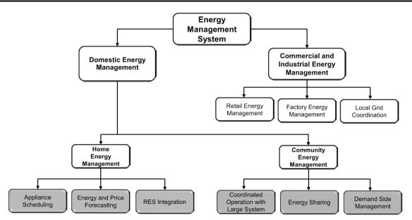
Figure 1. Energy management system in the smart grid system [8].
