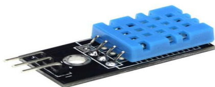
Fig.8 Humidity and Temperature Sensor
