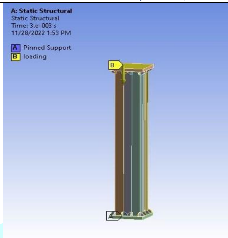
Fig 3.7 Application of loads in T section
