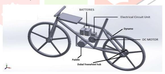
All the designed components and materials such as, bi-cycle, motor, dynamo, dual freewheel, chain sprockets, paddle, etc. were procured separately. Sub-assemblies was fabricated separately and finally all sub-assemblies was assembled as per cad model. The motor was controlled by the throttle.
