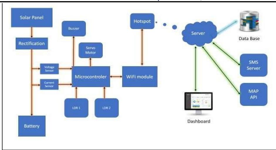
Figure 3. Digital control System for Solar Power Using IOT
