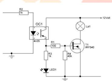
Fig -8 5V DC to 12V DC Drive Card circuit
