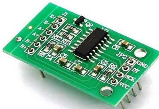
Load cell is connected with HX711 Load cell Amplifier using four wires. These four wires are Red, Black, White and Green/Blue. There may be slight variation in colors of wires from module to module. Below the connection details and diagram:
