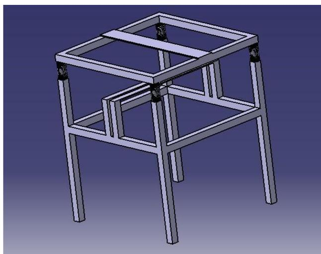
**Figure ; loadcell with driver seat unit.**
