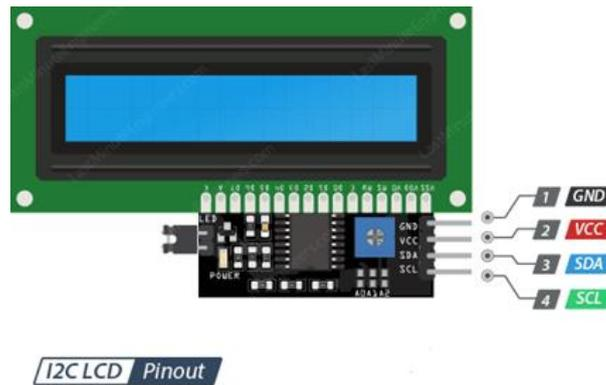
**GND** is a ground pin. Connect it to the ground of the Arduino.
