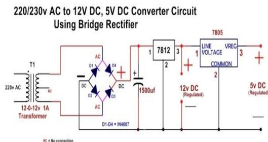
**Fig -10 Regulated Power supply unit**
