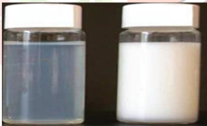
fig 1: picture of Nano emulsion (left) of size 35 nm and micro emulsion (right) of size 1 \mu m. [4]
