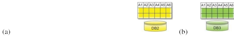
FIGURE 12. Data distribution. (a) centralized data. (b) horizontally partitioned data. (c) vertically partitioned data.
