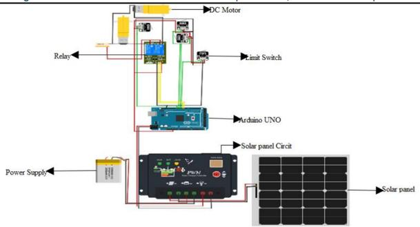
Circuit Diagram of proposed system connection consists of Solar panel, DC motor, Limit switches, Arduino Uno Board and power source as shown in the figure 2.
