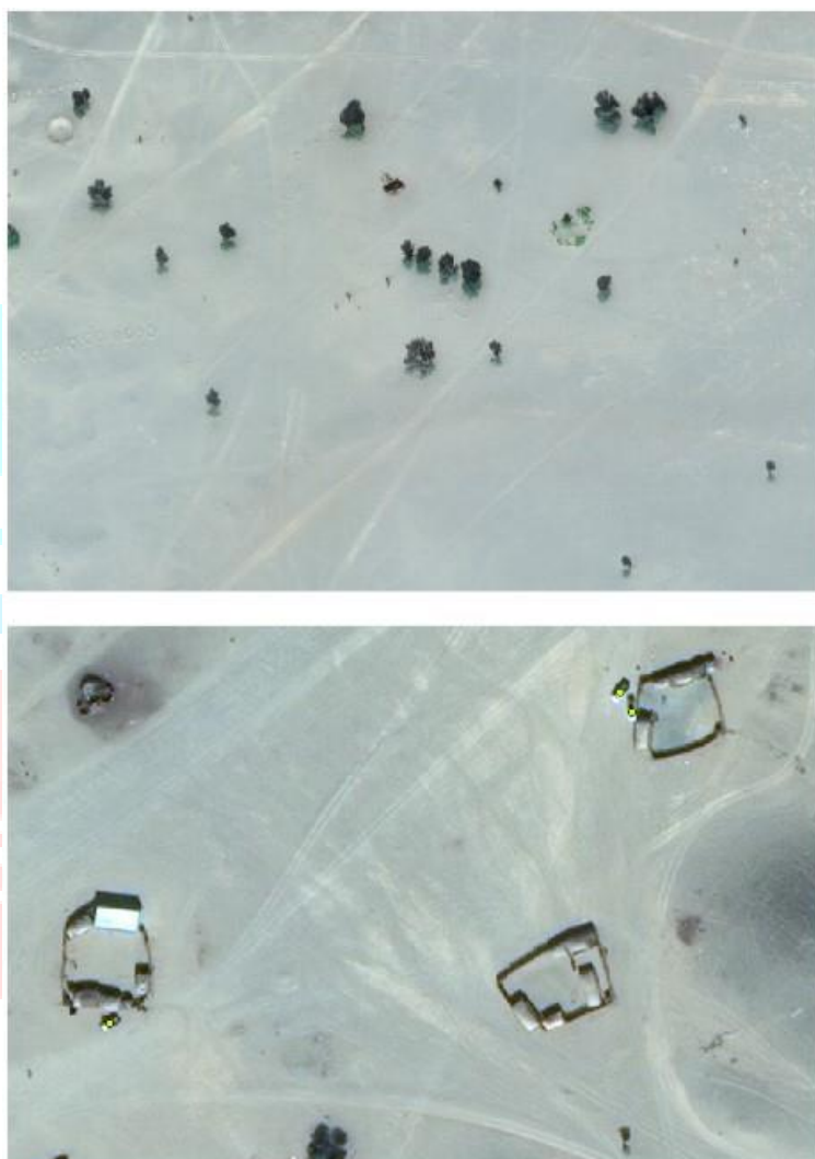
Fig. 7. Hard exemplifications in the desert terrain testing set where numerous objects can be confused with vehicles. Top illustration of small trees that look analogous to vehicles. nethermost illustration of veritably small structures that look analogous to vehicles( unheroic points are the vehicles in the ground verity).
