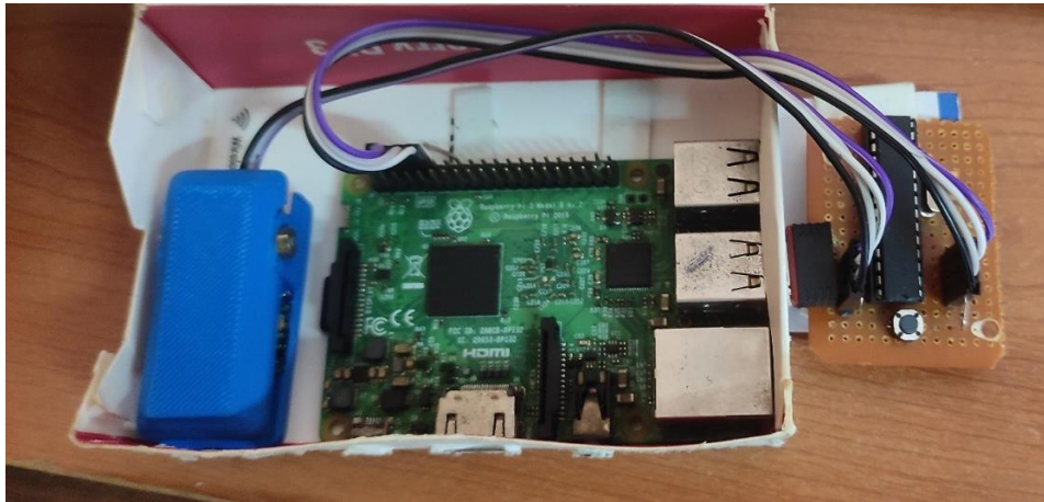
Fig 2: Hardware Implementation of Health Care system using raspberry pi
