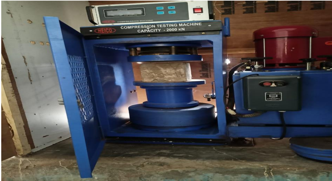
Figure no.1 Compressive strength testing
