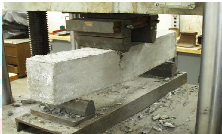
Figure 5. Flexural test setup
