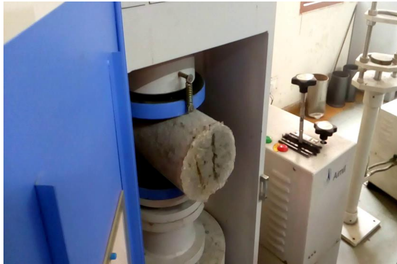
Image 7. Splitting tensile setup
