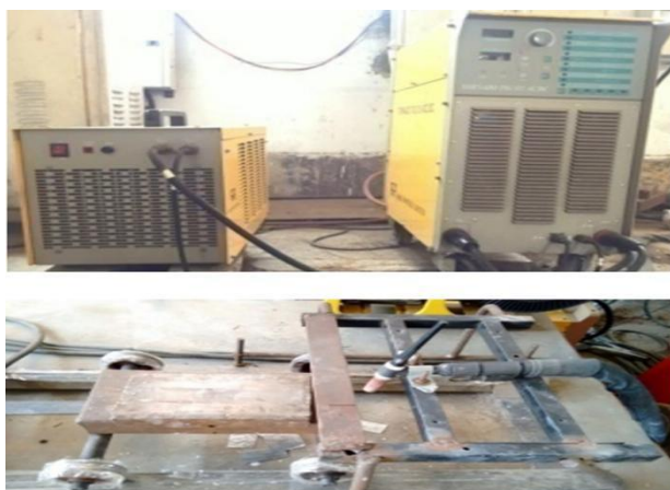
Fig: 2.1 TIG welding machine with special fixture.
