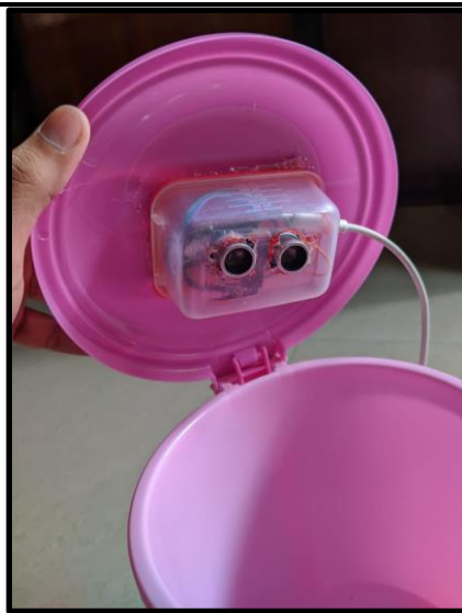
Ultrasonic sensor mounted on the dustbin
