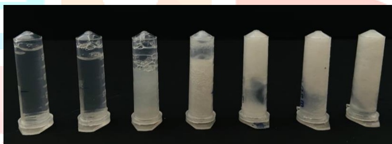
Fig 3. Hydrogel formation with increasing concentration of \beta -cd in SDS
