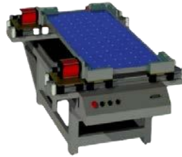
Figure 7: Auto Framing Machine
