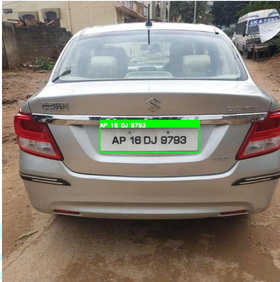
Fig.14: Indian car license plate detected and recognized.
