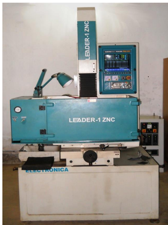
Fig. 2.1: Die Sinker EDM, Brand : Electronica Elektra Plus; Model : PS 50ZNC
