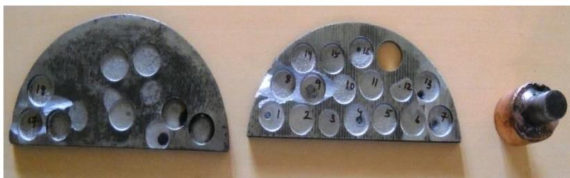
Fig. 3.1: Copper electrode and AISI P20 work-piece
