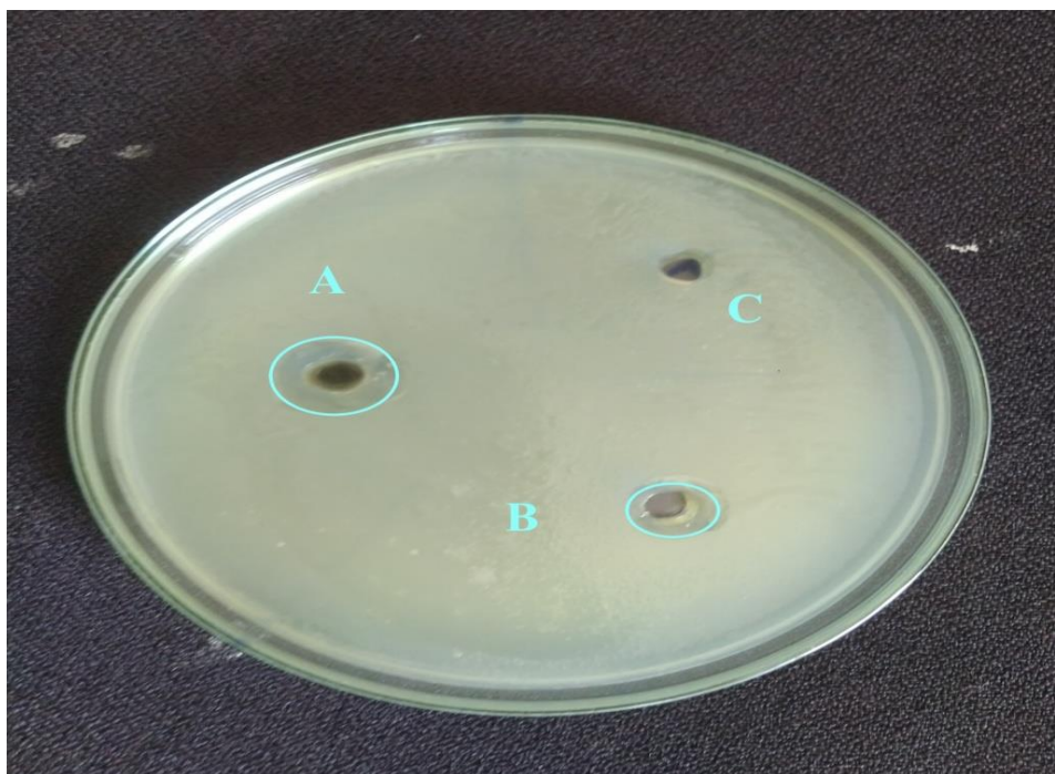
Fig. 3.13 Zone of inhibition shown by A. Nanoemulgel B. Gel C. control for S. aureus
