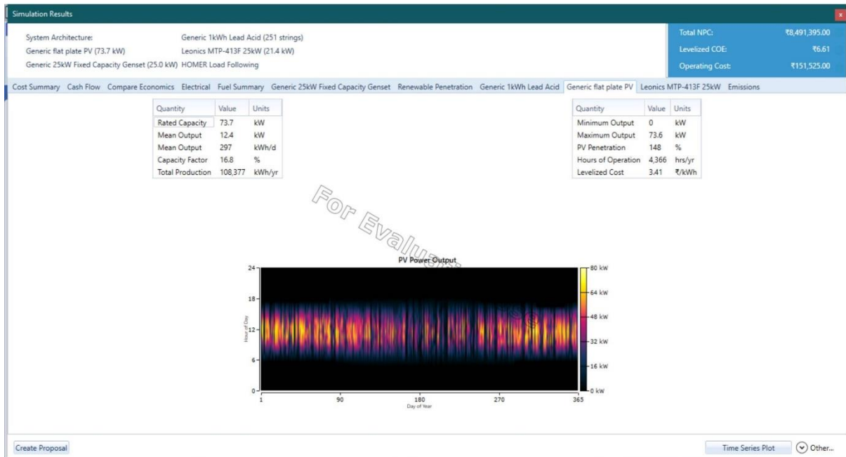
fig 14: PV power output
