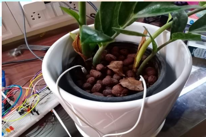
Figure 1: Electrodes inserted into the soil to make contact with the roots
