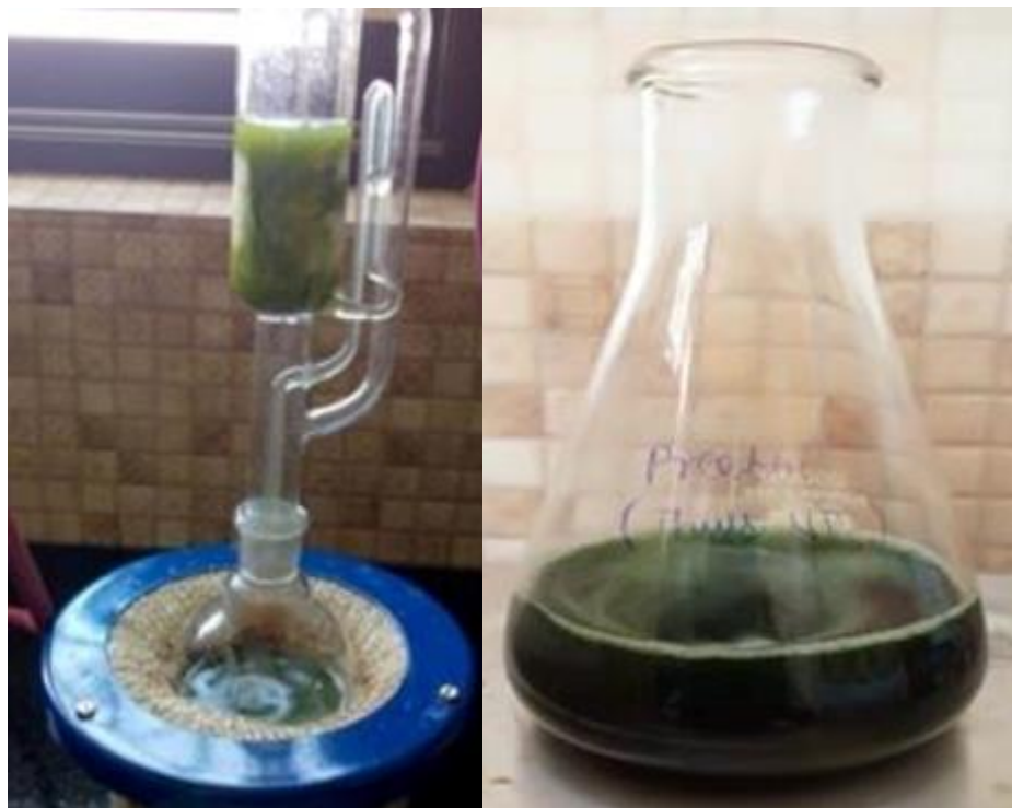
Fig no 1 – Extraction assembly & Extract photograph
