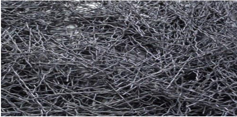
Figure 1.3 Steel fiber reinforcement
