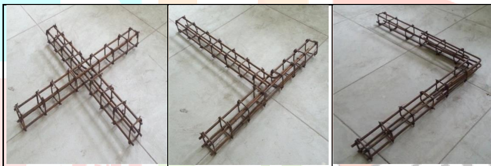
Figure 1.2 Beam column joint reinforcement
