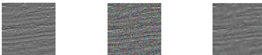
(a) Original seismic data (b) Seismic data after noise addition (c) Seismic data after noise reduction by DUDnCNN
