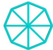
Fig. Radial Bracing
