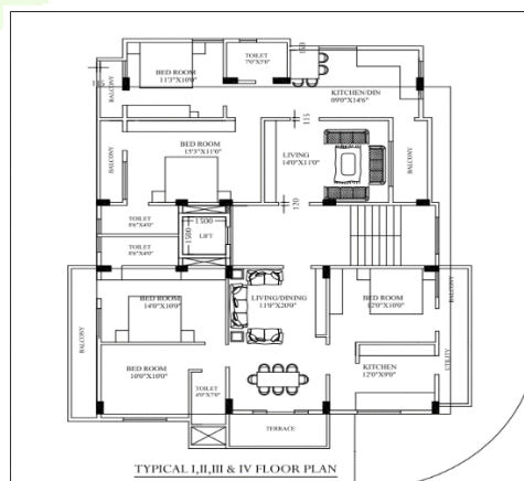
1:100 PLAN SHOWING COLUMN POSITIONS
