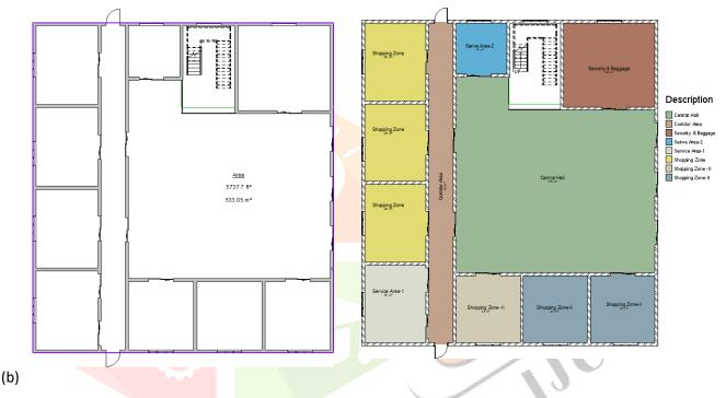
Figure 1a. The Gross Floor Plan area of 514m<sup>2</sup> and 1b. Description of floor area for utilization
