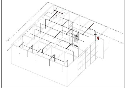
Figure.4 Typical arrangement of Fire Sprinkler system
