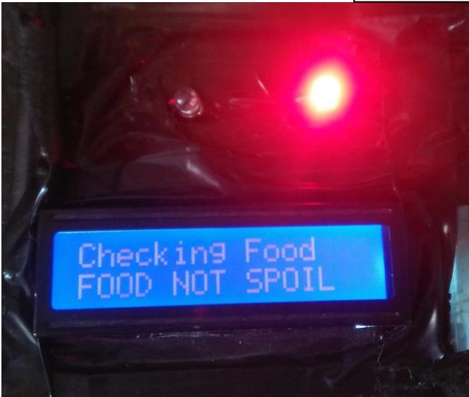
Food item checked and the system gives output that it is not spoiled.
