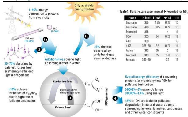
Figure:1-Detailing the low-energy conversion efficiencies in typical TiO<sub>2</sub> photocatalytic water treatment processes. Photons are generated either by electrical conversion or directly harnessing solar energy. (1a) Although low-pressure mercury lamps are typical, blue/UVA LEDs are being increasingly studied, with wall plug efficiencies nearing 30%. [Khan, A.; Balakrishnan, K.; Katona, T. Ultraviolet light-emitting diodes based on group three nitrides. Nat. Photonics 2008.]
