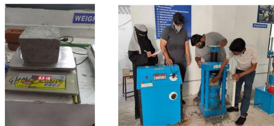
Fig: weighing the Block & Compressive strength testing (2000KN)
