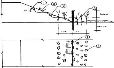
Fig. 25: Erosion of side slope by wave action
