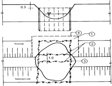
Fig. 35: Repair during low flow condition (water level differences of < 10 cm)
