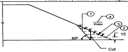
Fig.23: Cutting at side slope of embankment
