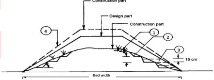
Fig. 21: Excessive subsidence of embankment crest and slope
