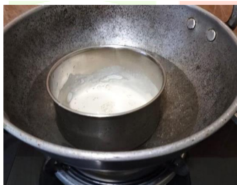
Figure 1: Double boiling method of natural soil mineral-Kaolin clay
