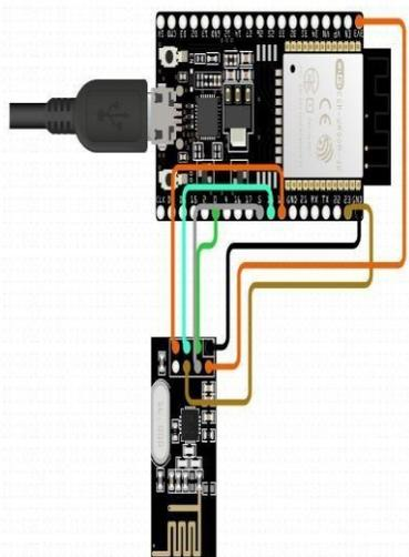
Fig. 5. Receiver Component Circuit Diagram
