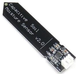
Fig. 4. Capacitive Moisture Sensor
