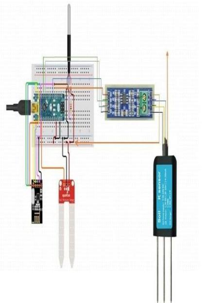
Fig. 2. Sender Component Circuit Diagram
