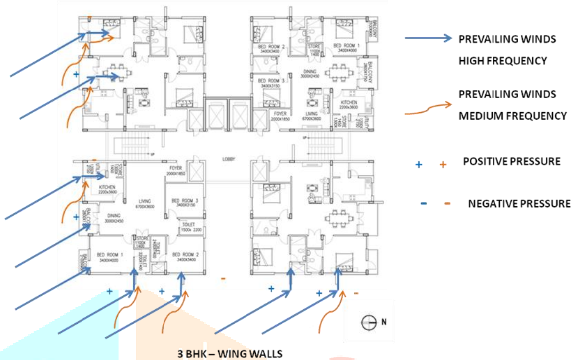
Figure 7- 3 BHK Typical floor plan showing Wing wall
