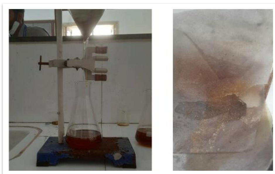
Fig. 1: \text{Na}_2\text{SO}_4 crystals and impurities on filter paper
