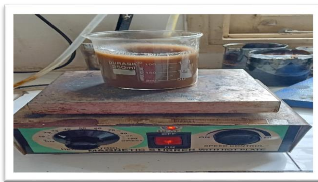
Fig3.4.2.2 the gelatinized potato peel waste on magnetic stirrer with hot plate
