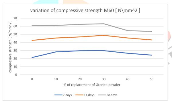
COMPRESSIVE STRENGTH OF M60 CONCRETE [N\mm^2]
