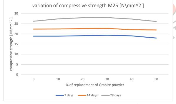
Compressive strength of M25 concrete [N\mm^2]
