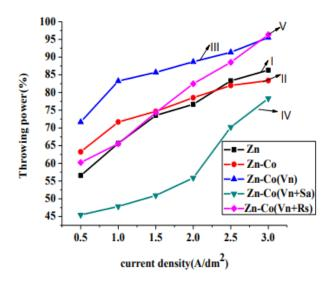
Figure 2- Graph of Throwing power v/s current density for Zinc and Zinc alloys as anodes. (18)
