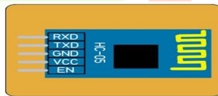
Figure 4 HC-05 Bluetooth Module
