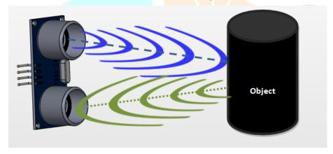
7. Working of Ultrasonic sensor HC-SR04
