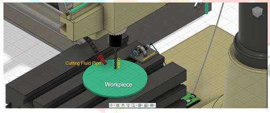
12. Schematic layout of sensor and cutting fluid pipe
