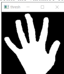
Fig 7: Front end window that shows the thresholded version of the input gesture
