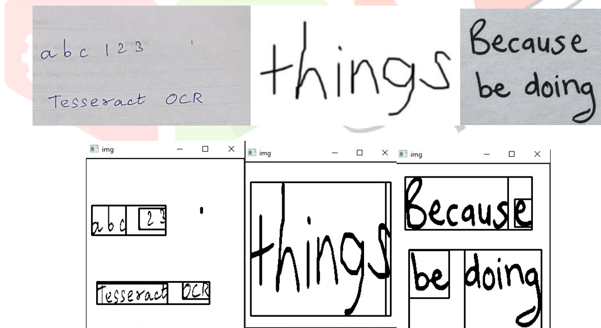
Fig 13,14,15 show the input handwritten text & Fig. 16,17,18 gives the filtered image with boxes around text
