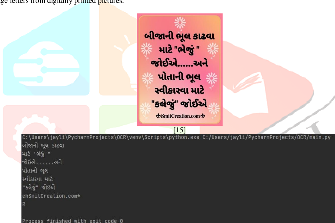
Fig 20 & 21 Input image having text in Gujarati with the corresponding output containing machine-readable text
