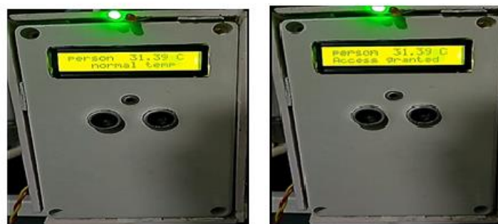
Figure 5: person's temperature being normal and granting access
