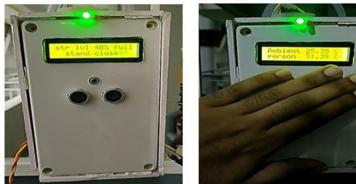
Figure 3: Indicating sanitizer level and detected a person
