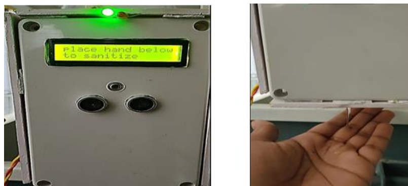
Figure 6: place hand below to sanitize message display and dispensing sanitizer
