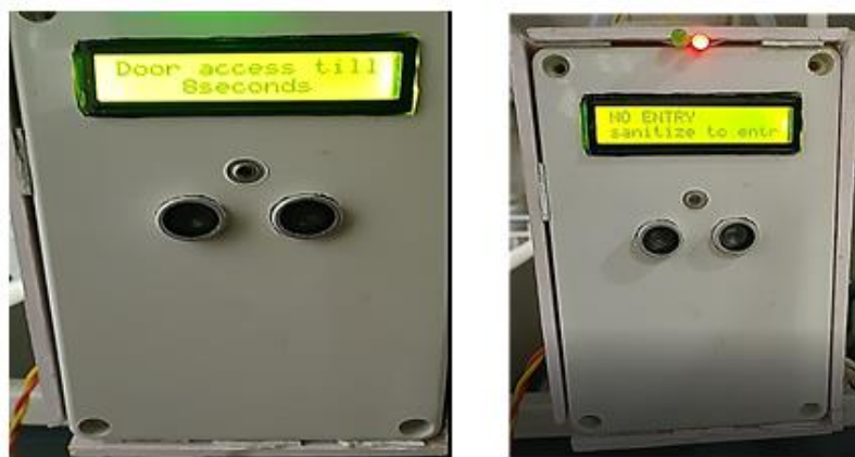
Figure 7: door access duration and denying access
