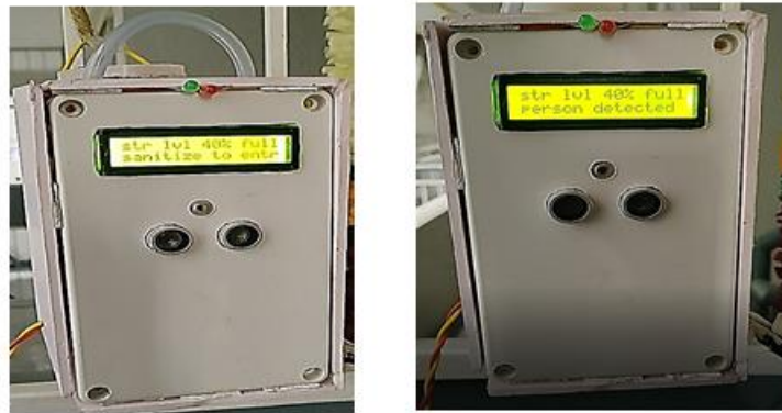
Figure 3: Indicating sanitizer level and detected a person
