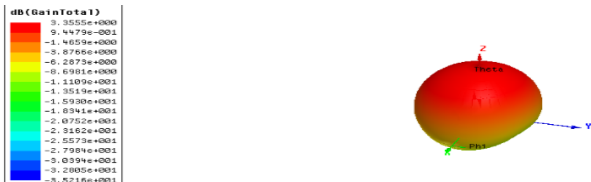
Fig 7: Gain for the V slot Hexagon Shape Stacked Patch Antenna at 1.6GHz
