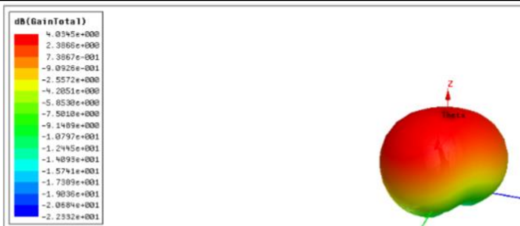
Fig 14: Gain for the Hexagon Shape Stacked Patch Antenna at 2.27GHz
