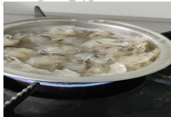
Fig No:4, The Fishscales soaked in NaOH soln is then Heated.
