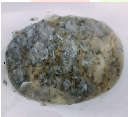
Fig No:3, Image of fish scales soaked in NaOH Soln.
