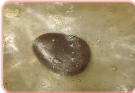
Fig No 9: Bio Plastic Film Obtained from Fish Scale is wrapped in a candy.
