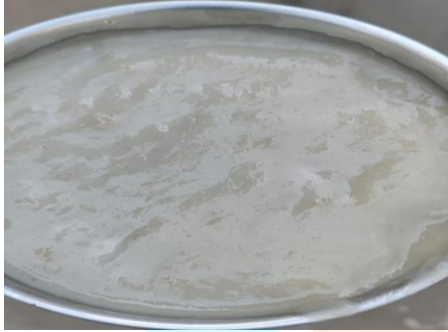
Fig No:7, The Prepared Bioplastic is sheeted in the tray for drying.
