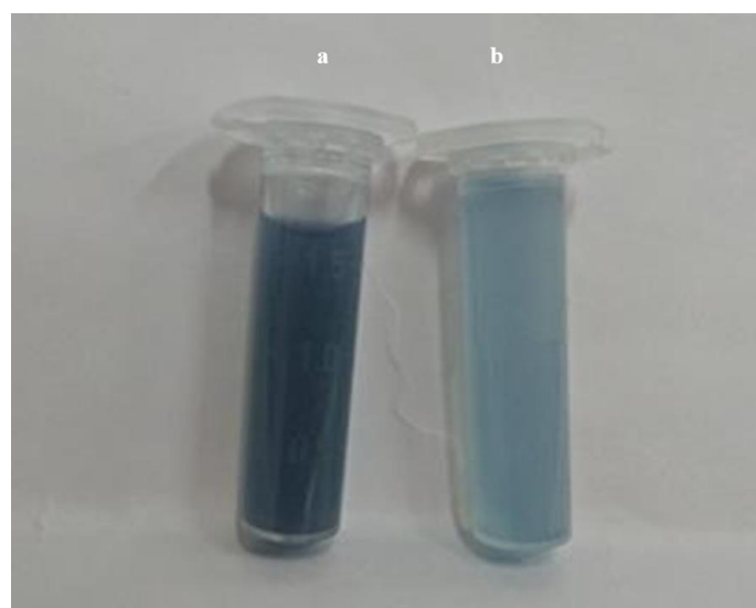
Figure 8. Estimation of anti-oxidant capacity of C – Phycocyanin by DPPH assay
